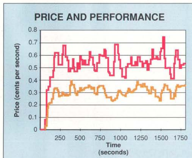
Figure 3: The price of computing time on different machines is different if the machines have different capabilities. The dark line shows the price of time (established by auction) on the faster and consequently more valuable Sun-4/260. The gray line is the price of computation on a Sun-4/100.
